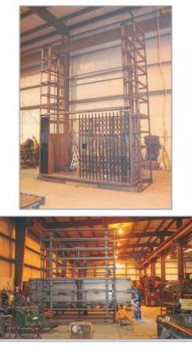
Double Frame Vertical Reciprocating Conveyors are specifically designed for vertical movement of a large, bulky, heavy material from one elevation to another. Requires minimal floor space and easily installed. The model RJS-2 can be surface mounted or placed in a shallow pit. Our RJS-2 model comes with all the same safety features as the RJS model. The RJS-2 has 2 pistons each with dual ANSI chains.
