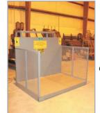
48" high expanded metal guards on non-access sides
