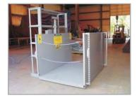
48" high solid guard on non-access sides dual safety chains on access sides
